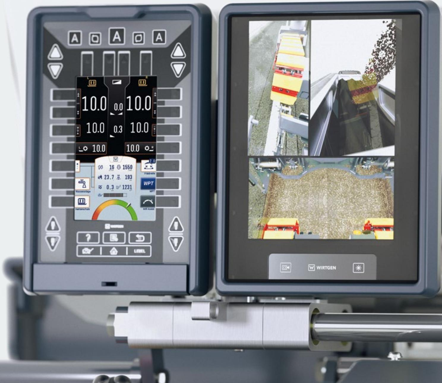
**01** 10" control panel with split screen for the simultaneous display of multiple camera images.
