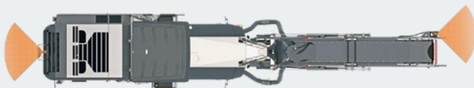
**Two-Camera System:** Rear-view camera / material loading camera
